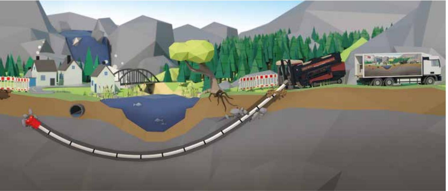
WEIGAND Bau specializes in laying fiber optic cables in rough terrain. Horizontal Directional Drilling (HDD) technology enables the trenchless laying of cables: under streets, buildings, and waterways.
